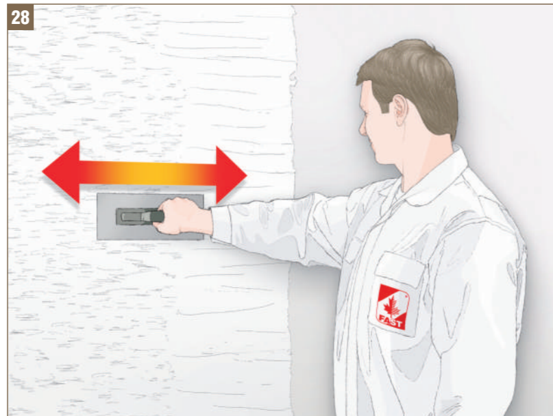
Fig. 28 - Giving texture to plaster - horizontal grated structure © FAST 2008
