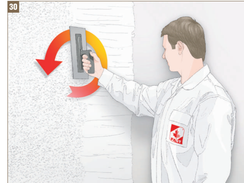
Fig. 30 - Texturing plaster - "fleece" structure © FAST 2008
