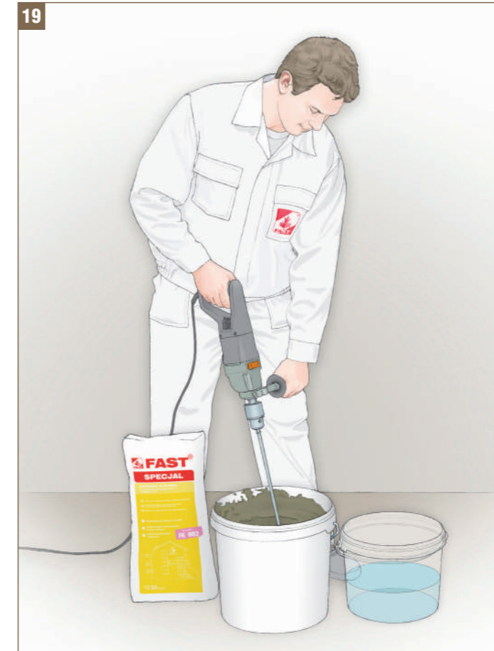
Fig. 19 - Preparation of FAST SPECJAL mortar glue © FAST 2008
